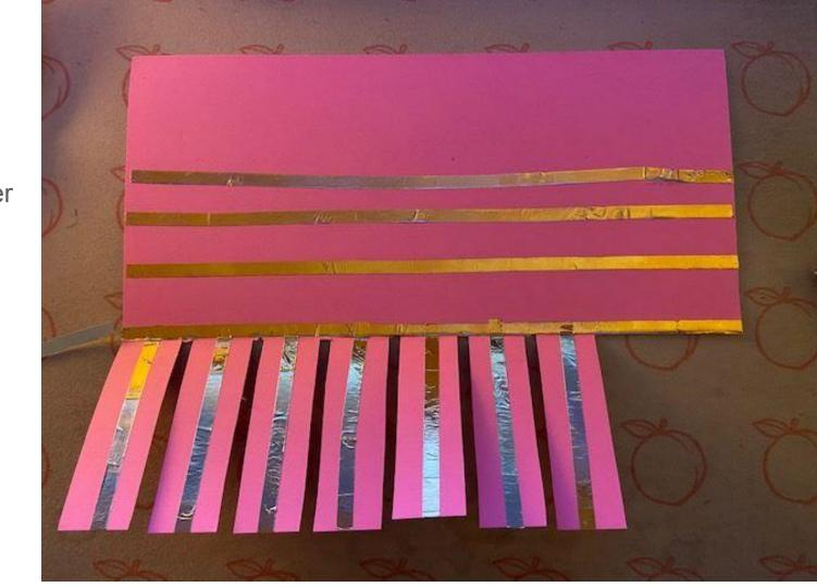
Glue pieces of paper over sections of the copper tape to create our binary pattern
