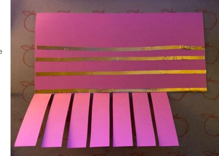
Place shorter strips of copper tape on the underside of the keys
