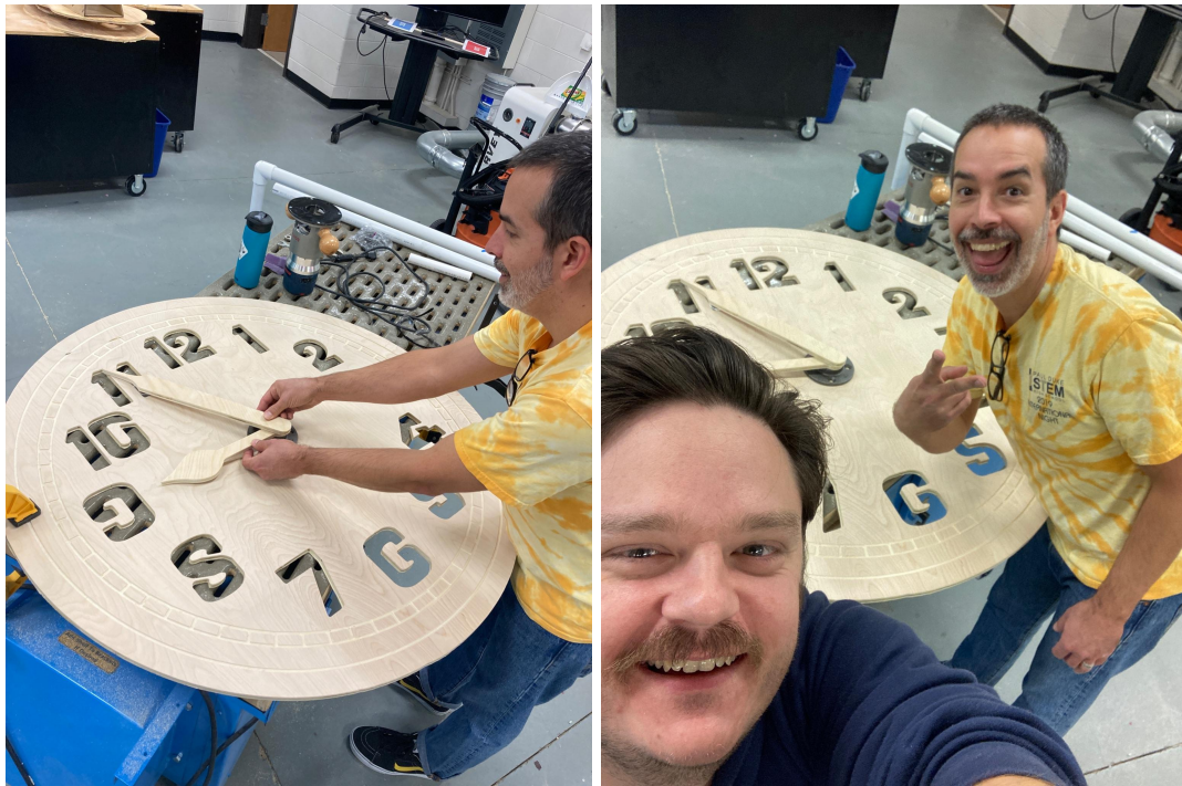
Mr. Cochran and I decided to use \frac{1}{4} " thick sanded plywood. The Foamular seemed a bit too fragile for the scale we needed. The final results were much better than the Foamular version.
