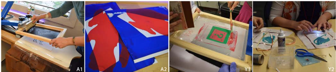
Figure 1. Screenprinting with conductive ink and thermochromic prints on paper developed during our art workshop with adults (A1 & A2); children screenprinting and assembling foldable circuits on fabric during our STEAM class for junior highschool youths (Y1 & Y2).
